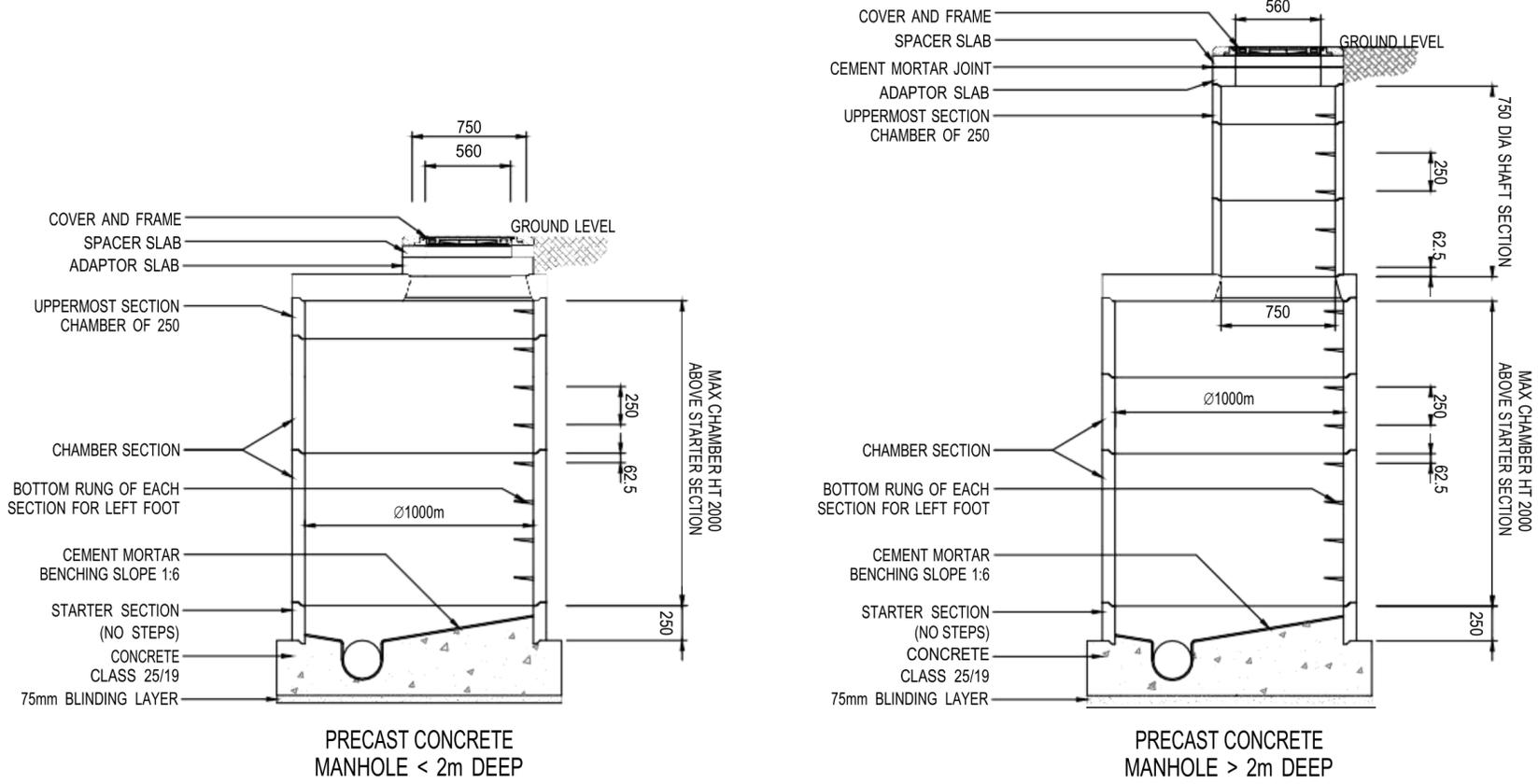
TYPICAL SEWER MANHOLE DETAIL
