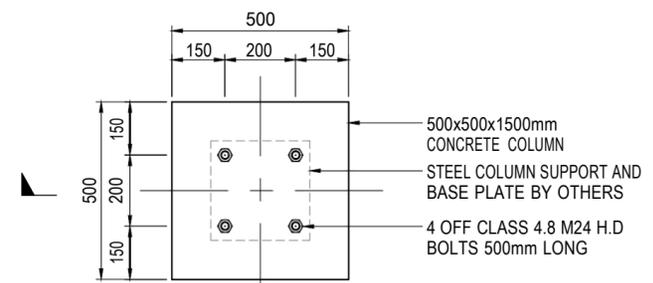
**PLAN CONCRETE STUB C-F-01**
